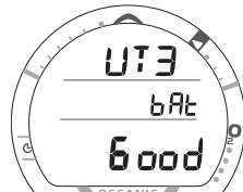
Fig. 4 - Battery Status (Good)
