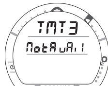
Fig. 6 - Transmitter 3 Status (Not Available)
