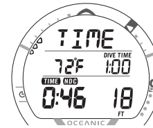
Fig. 120 - FREE DIVE MAIN (During EDT ALARM)
