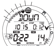
Fig. 80 - NORM DELAYED VIOLATION #1 MAIN
